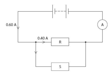
i R has a resistance of 11 ohms.Calculate the potential difference across R.
