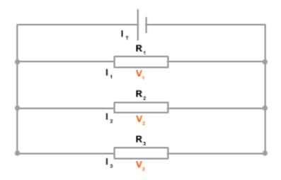
**a i**  $R_1$  has a resistance of 5 ohms. The current flowing in it is 2A. Calculate the potential difference across  $R_1$ .
