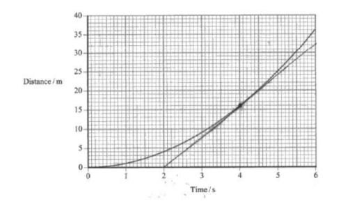
(a) Use the distance-time graph to determine the speed of the object at a time of 4.0 s.
