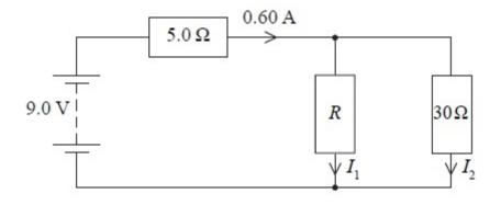
**a** Calculate the potential difference across the 5  $\Omega$  resistor.
