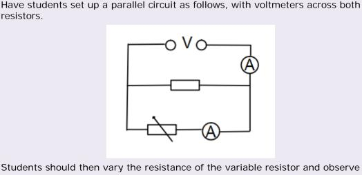
Students should then vary the resistance of the variable resistor and observe what happens to the voltage on both voltmeters and the current in both ammeters. Once this has been discussed they should record both currents and the voltage for a range of variable resistor settings and work out the resistance of the variable resistor and total resistance of the circuit. They should then plot graphs of:
