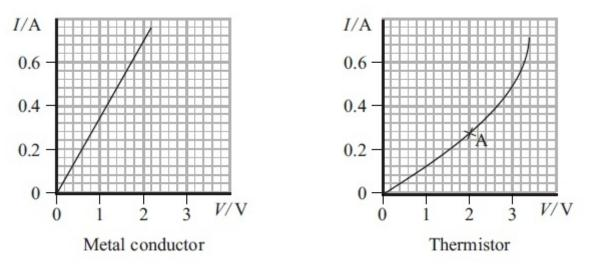
i Calculate the resistance of the thermistor at point A.
