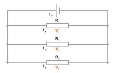
**a)** i  $R_1$  has a resistance of 5 ohms. The current flowing in it is 2A. Show that the potential difference across  $R_1$  is 10V.
